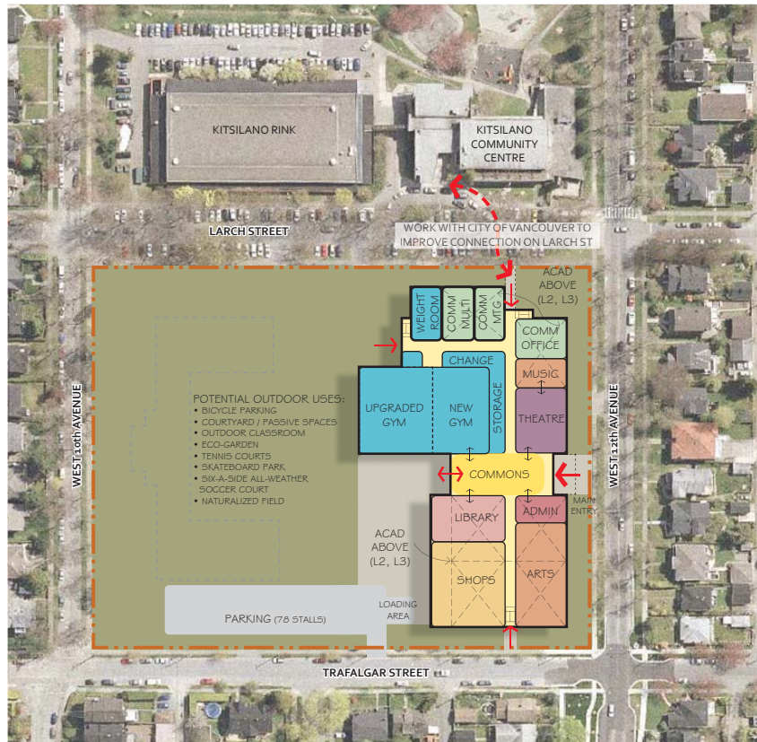
Concept F proposes a completely new three-storey school to be constructed along 12th Avenue, reusing the existing large gym and demolishing all other existing buildings.
