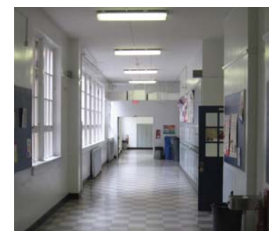
• Intense natural lighting in single loaded corridor along north side of the building
